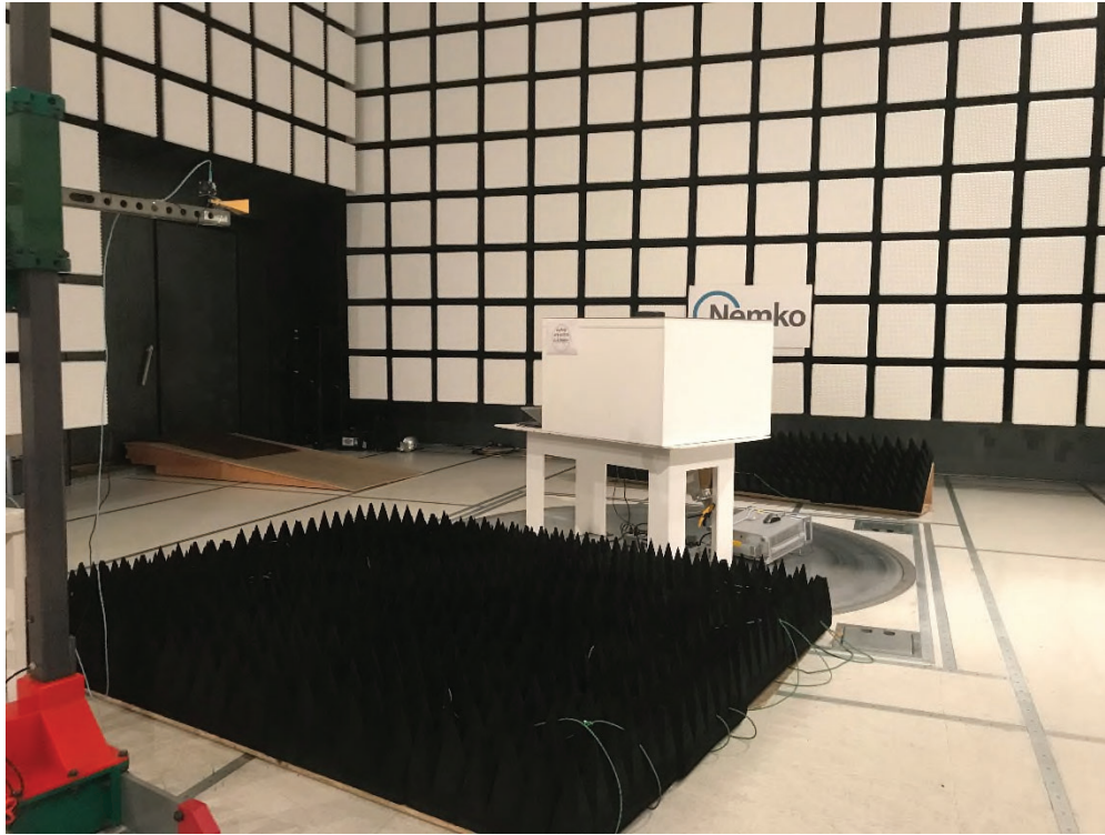
Figure 8.1.12 Radiated emissions setup from 18 - 40 GHz
