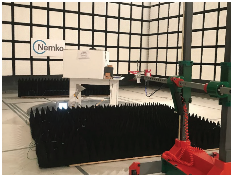
Figure 8.1.10 Radiated emissions setup from 30-1000 MHz
