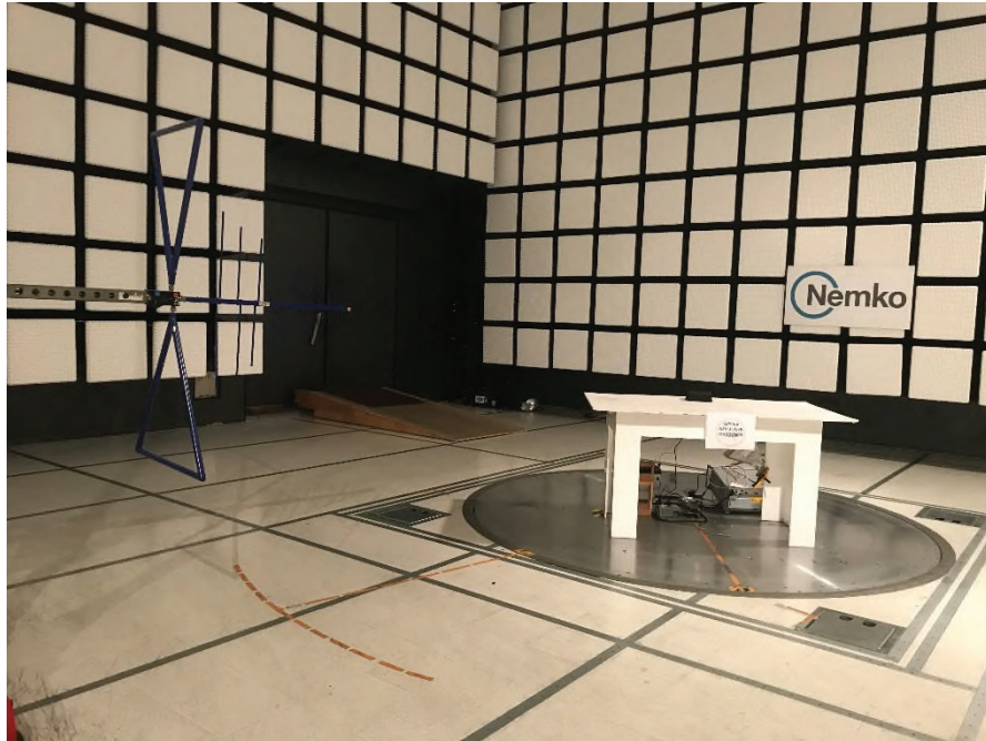
Figure 8.1.10 Radiated emissions setup from 30-1000 MHz
