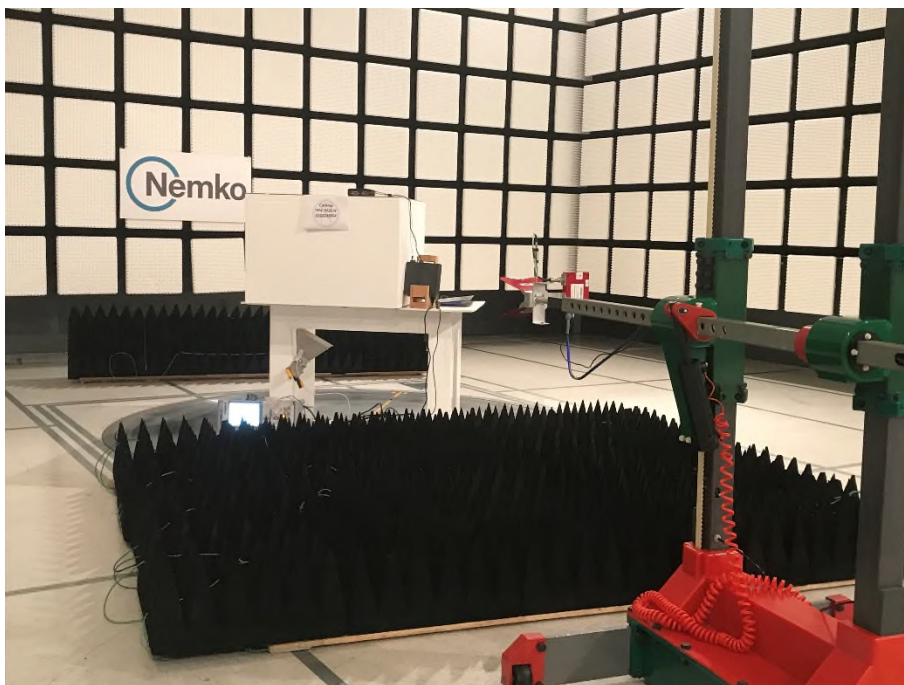
Figure 8.1.10 Radiated emissions setup from 30-1000 MHz
