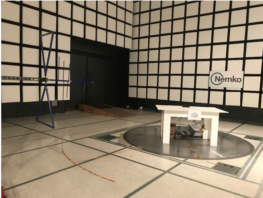
Figure 8.1.10 Radiated emissions setup from 30-1000 MHz
