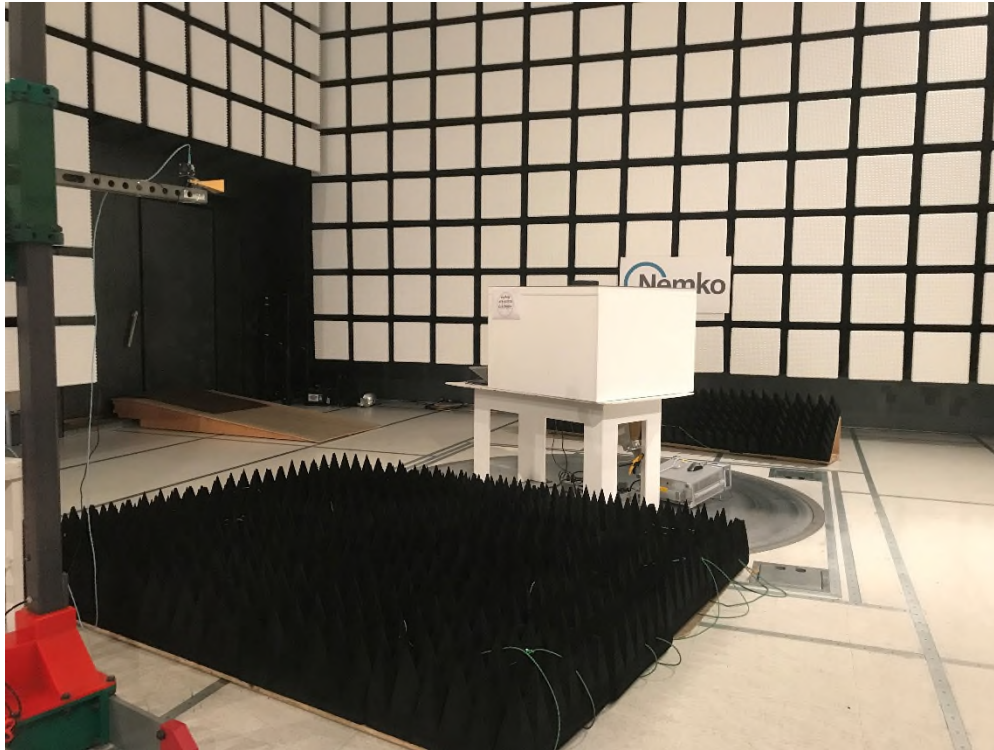
Figure 8.1.12 Radiated emissions setup from 18 - 40 GHz
