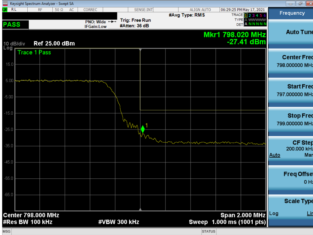
Plot 7-14. Upper Band Edge Plot (LTE Band 14, 5MHz QPSK - RB Size 25)
