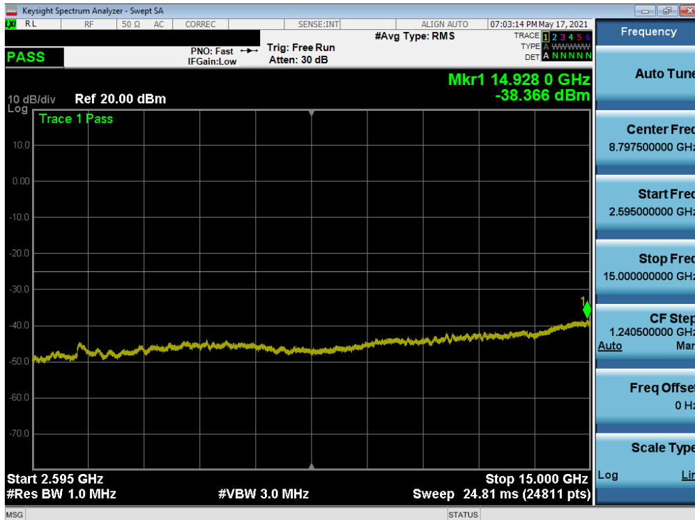
Plot 7-16. Conducted Spurious Plot (LTE Band 7 - 20MHz QPSK - RB Size 1, RB Offset 0 - High Channel)
