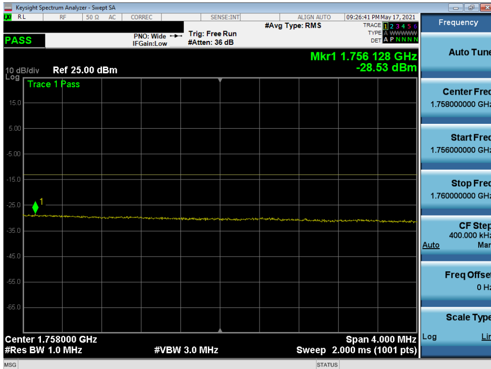
Plot 7-69. Upper Extended Band Edge Plot (LTE Band 4 - 20MHz QPSK – Full RB)
