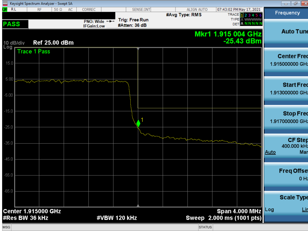
Plot 7-71. Upper Band Edge Plot (LTE Band 25 - 3MHz QPSK – Full RB)
