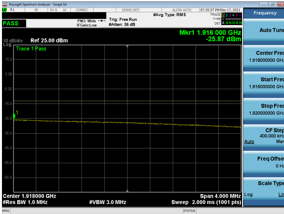
Plot 7-48. Extended Upper Band Edge Plot (LTE Band 25 - 20MHz QPSK – Full RB)
