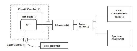
**Testing method:** Specified under each RF-Parameter test
