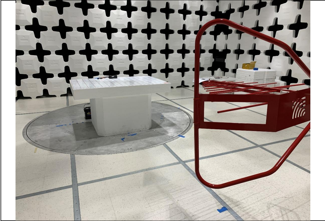
Radiated Emissions Below 1GHz setup – Front
