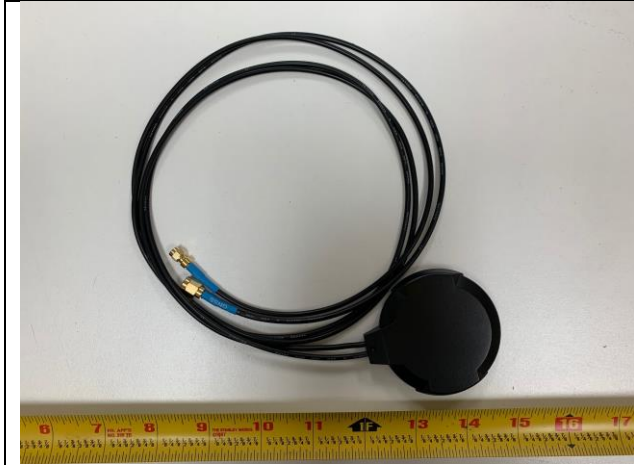
Cellular antenna - Top
