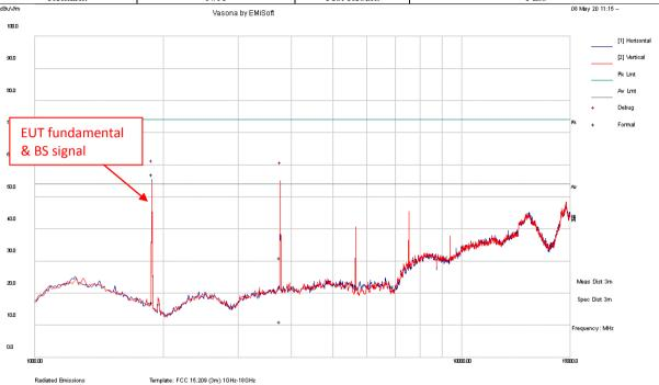
Margin Frequency Cable Level Measurement Hgt Azt Limit Raw dBuV AF dB Pol Pass/Fail MHz Loss dBuV/mType cm Deg dBuV/mdB 3760.5 31.3 -16.5 31.1 232 32 -42.9 Pass 16.4 Peak Max 74
