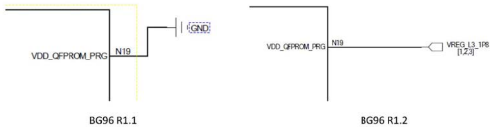
Figure 1: Schematic Designs of BG96 R1.1 and R1.2
