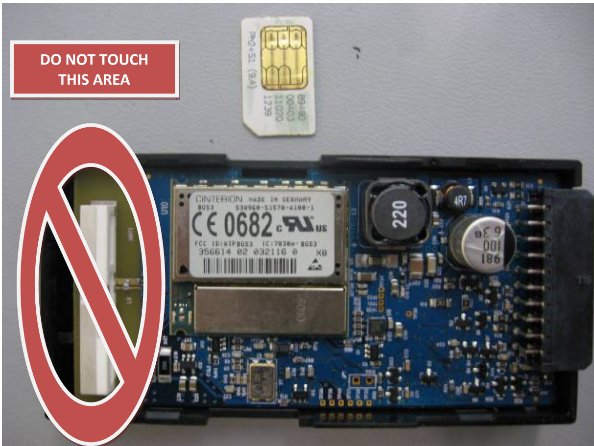
Figure 12 - LMU-2640™ SIM Alignment
