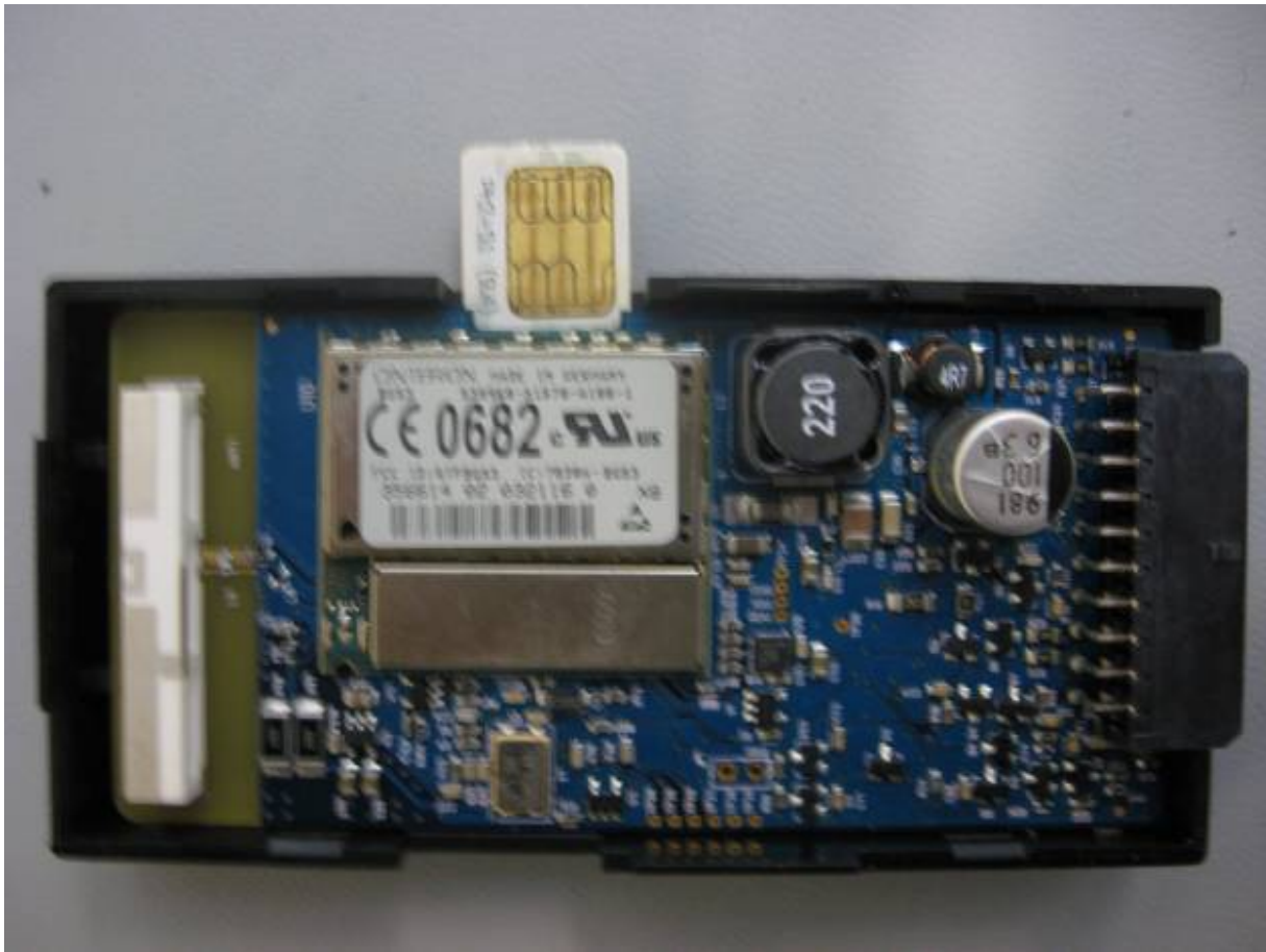
Figure 13 - LMU-2640™ - Partially Inserted SIM
