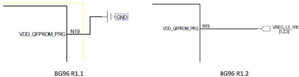
Figure 1: Schematic Designs of BG96 R1.1 and R1.2
