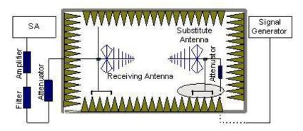
In the chamber, an substitution antenna for the frequency band of interest is placed at the reference point of the chamber. An RF Signal source for the frequency band of interest is connected to the substitution antenna with a cable that has been constructed to not interfere with the radiation pattern of the antenna. A power (P<sub>Mea</sub>) is applied to the input of the substitution antenna, and adjust the level of the signal generator output until the value of the
