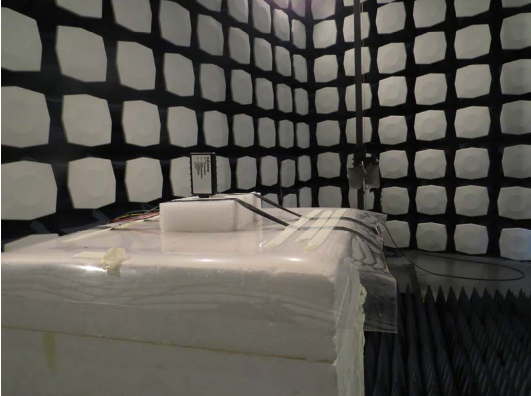
Picture 2: Radiated Spurious Emissions Test setup
