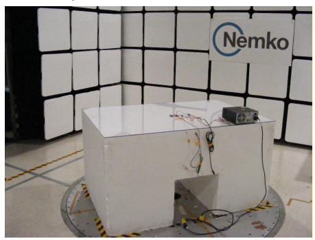
Figure 8.1-6: Radiated emissions 30 MHz-1 GHz Back Picture
