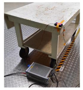
Figure 8.2-3: Conducted emissions 9 kHz – 30 MHz Side Picture
