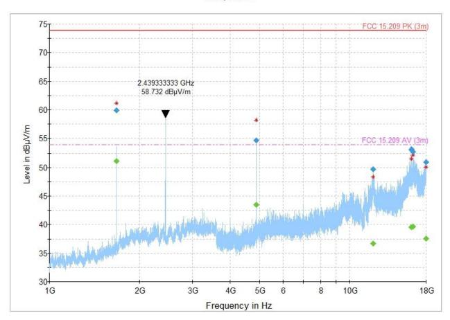
Figure 8.1-2: Radiated Emissions, 1 GHz to 18 GHz - GSM 850 (837 MHz), Bluetooth (2440 MHz) active Table 8.1-2: Radiated Emissions, 1 GHz to 18 GHz - GSM 850 (837 MHz), Bluetooth (2440 MHz) active
