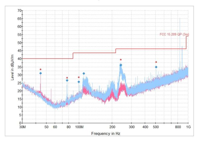
Figure 8.1-1: Radiated Emissions, 30 MHz to 1 GHz - GSM 850 (837 MHz), Bluetooth (2440 MHz) active
