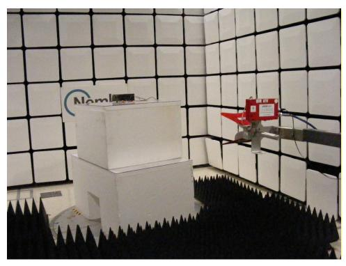
Figure 8.1-7: Radiated emissions 1 GHz-18 GHz - Front
