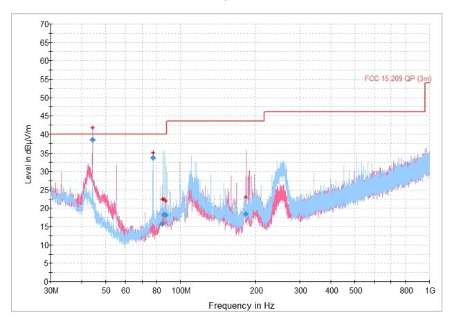
Figure 8.1-3: Radiated Emissions, 30 MHz to 1 GHz - GSM 1900 (1880 MHz), Bluetooth (2440 MHz) active Table 8.1-3: Radiated Emissions, 30 MHz to 1 GHz - GSM 1900 (1880 MHz), Bluetooth (2440 MHz) active
