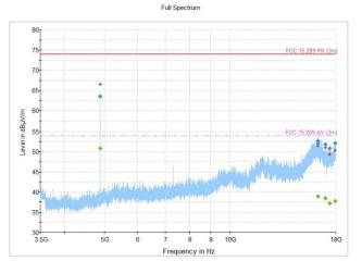
Figure 8.1-4: Radiated Emissions, 1 GHz – 18 GHz - GSM 1900 (1880 MHz), Bluetooth (2440 MHz) active
