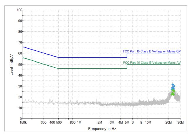
Figure 8.2-1: Conducted Emissions, 9 kHz - 30 MHz- GSM 850 (837 MHz), Bluetooth (2440 MHz) active
