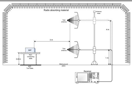
Figure 9.1-1 30 MHz - 1000 MHz Setup
