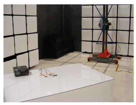
Figure 8.1-5: Radiated emissions 30 MHz-1 GHz Front Picture
