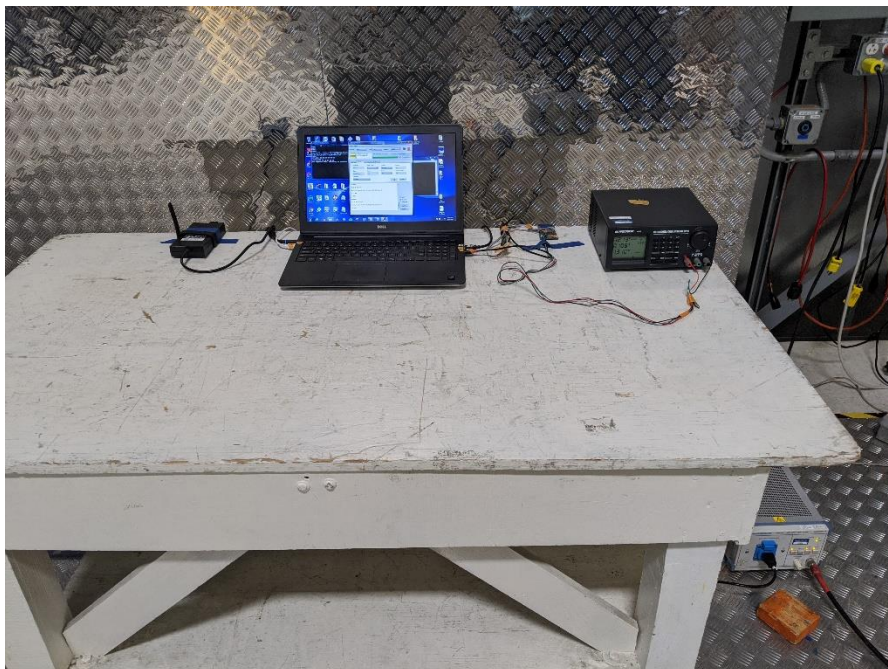
Figure 6 – AC conducted emissions test setup, front view
