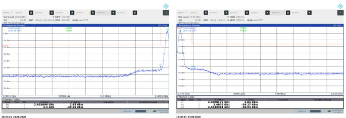
Figure 8.4-1: Conducted band edge measurement, 2402 MHz
