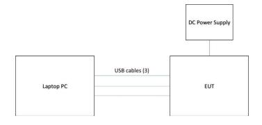
Figure 3.4-1: Test setup
