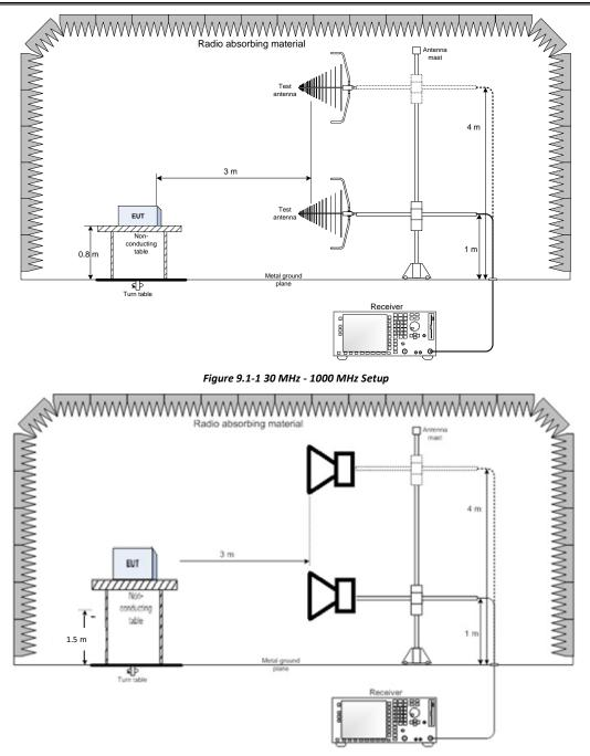
Figure 9.1-2 1 GHz - 26 GHz Setup
