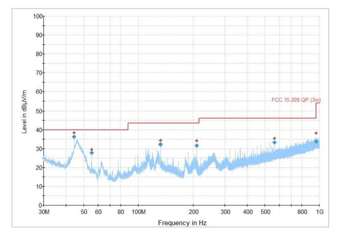
Figure 8.6-6: Radiated emissions, 2440 MHz, 30 – 1000 MHz
