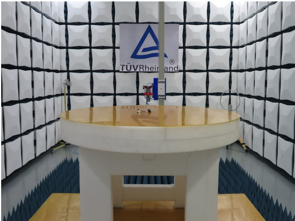
Photograph 2: Set-up for Radiated Spurious Emission, Above 1GHz
