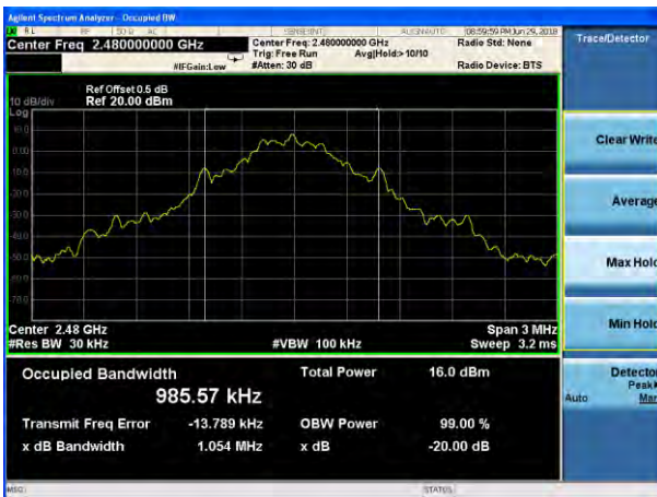
20dB Bandwidth plot on channel 78 (1Mbps)
