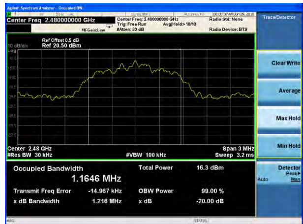
20dB Bandwidth plot on channel 78 (2Mbps)
