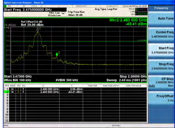
\pi /4-DQPSK: Band Edge-High Channel (Hopping Mode)
