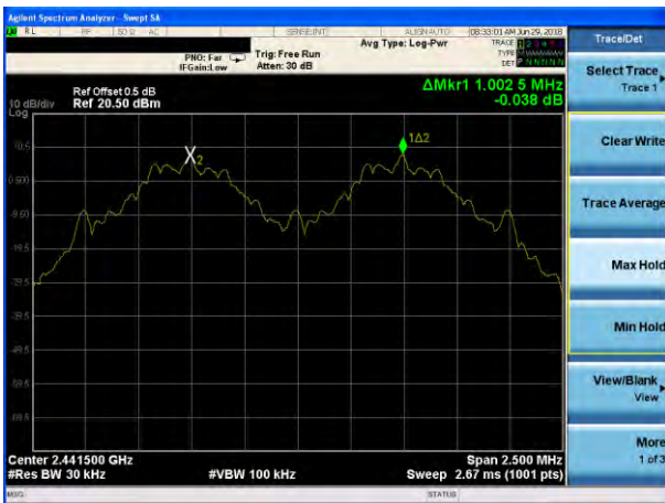
(1Mbps) Channel Separation plot on channel 39-40
