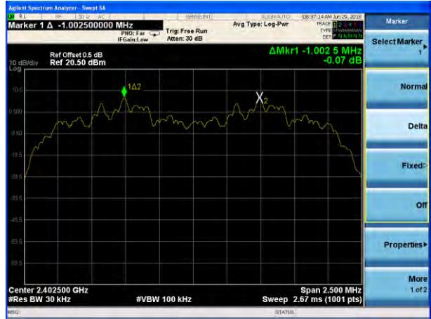
(2Mbps) Channel Separation plot on channel 39-40
