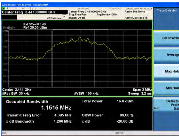
20dB Bandwidth plot on channel 78 (3Mbps)
