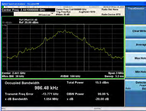
20dB Bandwidth plot on channel 78 (1Mbps)
