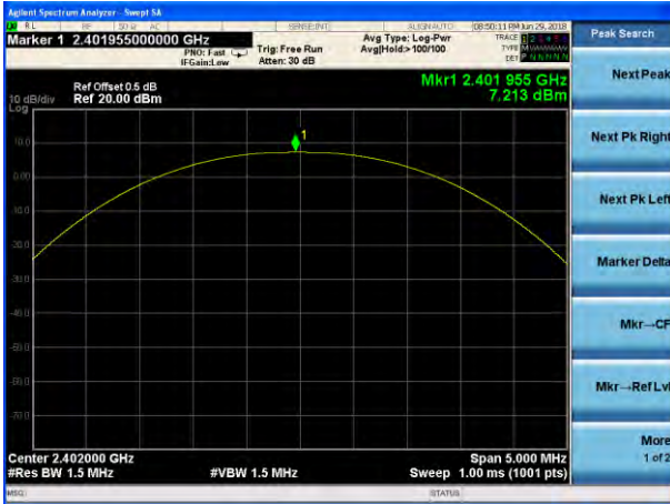
Peak output Power plot on channel 39 (1Mbps)
