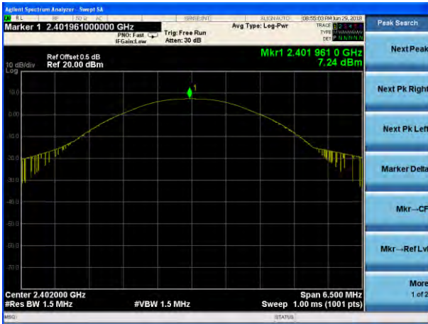
Peak output Power plot on channel 39 (3Mbps)
