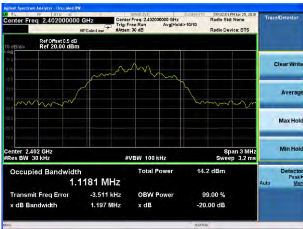
20dB Bandwidth plot on channel 00 (3Mbps)
