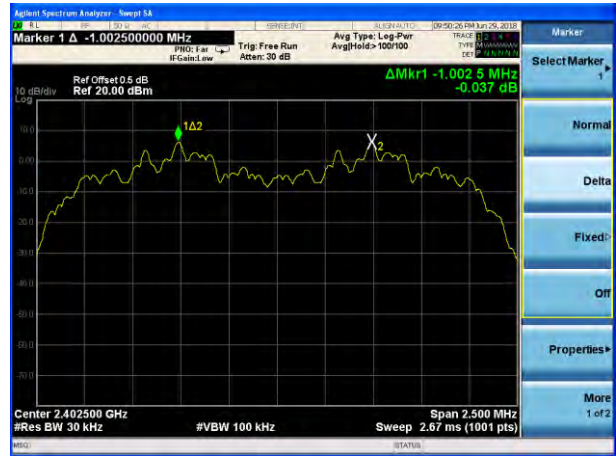
(2Mbps) Channel Separation plot on channel 39-40
