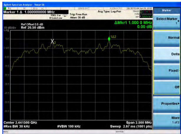
(2Mbps) Channel Separation plot on channel 39-40
