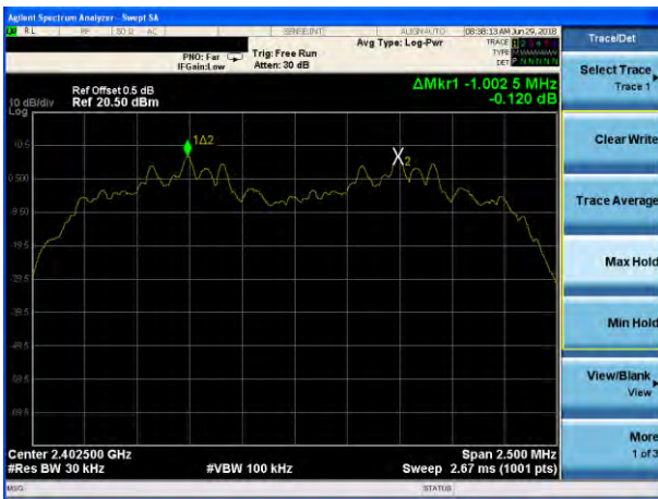
(3Mbps) Channel Separation plot on channel 00-01
