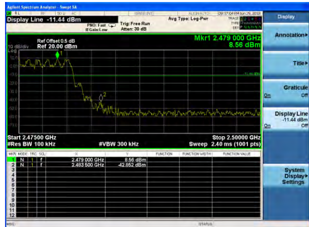
8-DPSK: Band Edge-High Channel (Hopping Mode)
