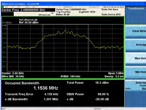
20dB Bandwidth plot on channel 78 (3Mbps)
