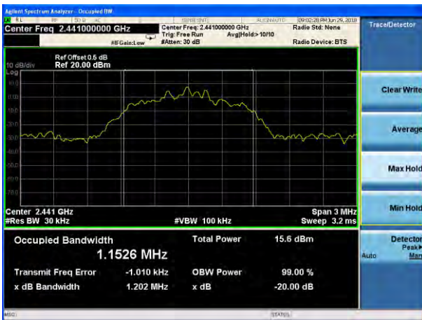
20dB Bandwidth plot on channel 39 (3Mbps)
