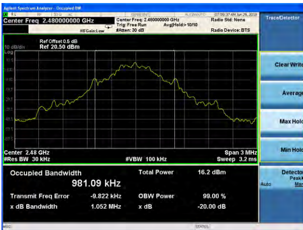
20dB Bandwidth plot on channel 78 (1Mbps)
