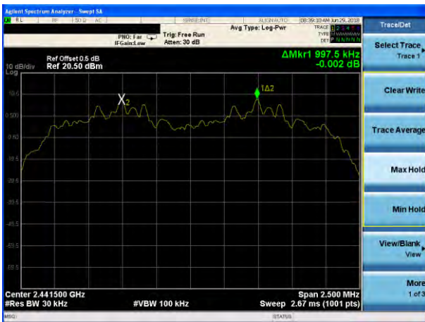
(3Mbps) Channel Separation plot on channel 39-40
