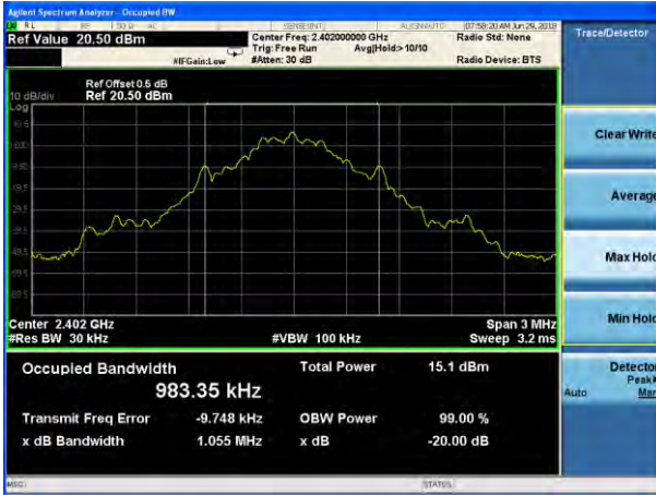
20dB Bandwidth plot on channel 39 (1Mbps)
