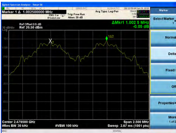
(1Mbps) Channel Separation plot on channel 77-78
