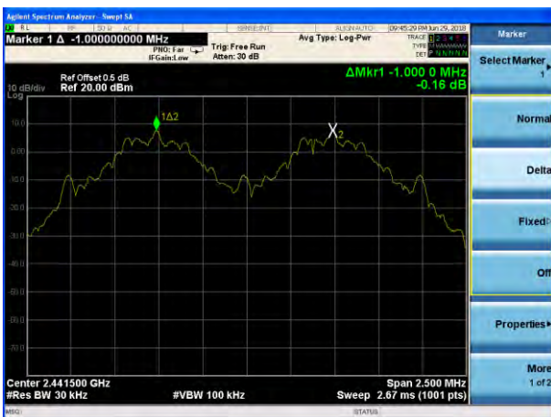
(1Mbps) Channel Separation plot on channel 39-40
