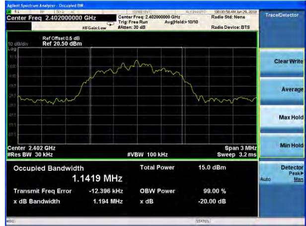
20dB Bandwidth plot on channel 39 (2Mbps)
