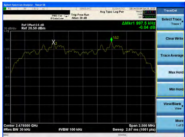
(2Mbps) Channel Separation plot on channel 77-78
