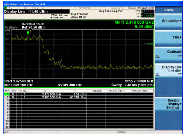
\pi /4-DQPSK: Band Edge-High Channel (Hopping Mode)
