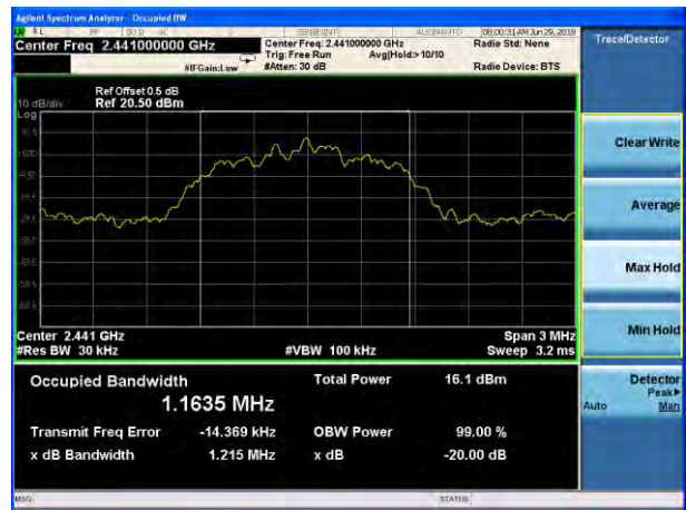
20dB Bandwidth plot on channel 78 (2Mbps)
