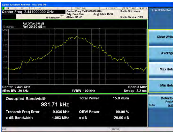
20dB Bandwidth plot on channel 78 (1Mbps)
