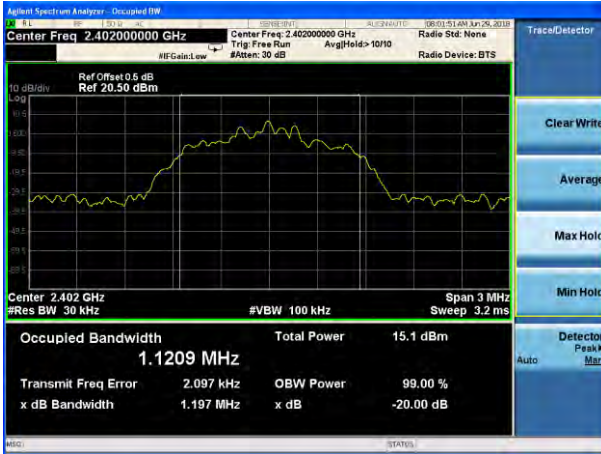
20dB Bandwidth plot on channel 39 (3Mbps)
