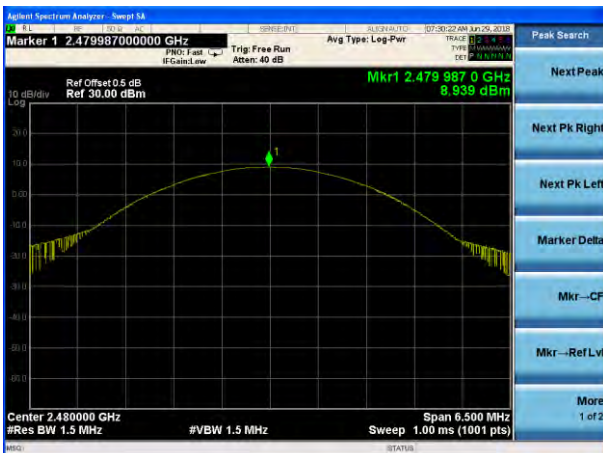
Peak output Power plot on channel 78 (3Mbps)
