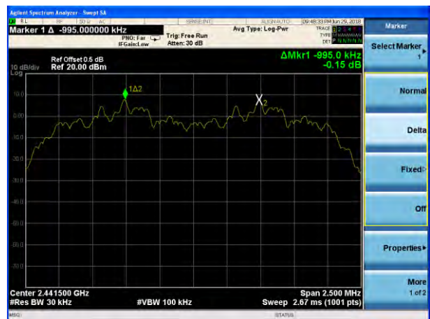
(2Mbps) Channel Separation plot on channel 39-40
