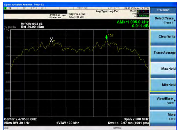
(2Mbps) Channel Separation plot on channel 77-78
