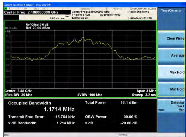
20dB Bandwidth plot on channel 78 (2Mbps)
