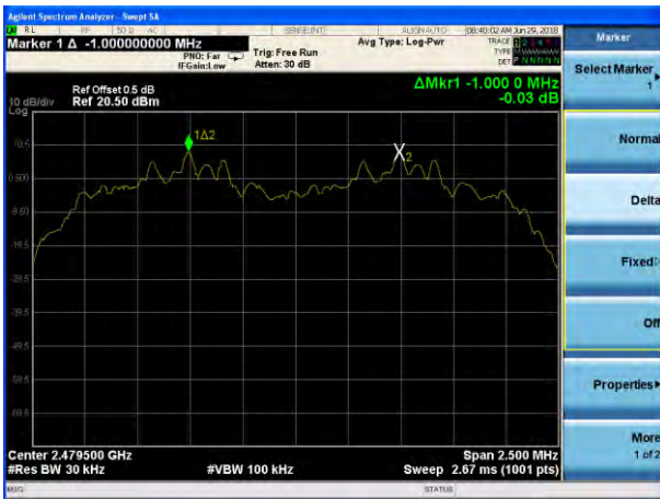
(3Mbps) Channel Separation plot on channel 77-78
