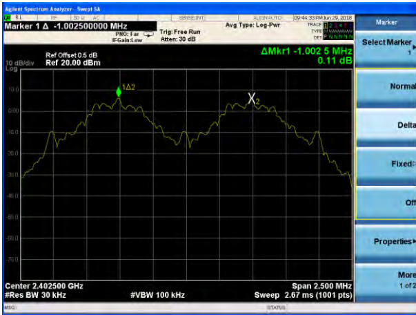
(1Mbps) Channel Separation plot on channel 39-40
