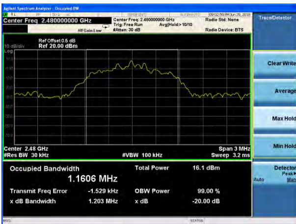
20dB Bandwidth plot on channel 78 (3Mbps)
