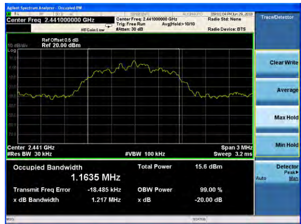
20dB Bandwidth plot on channel 78 (2Mbps)
