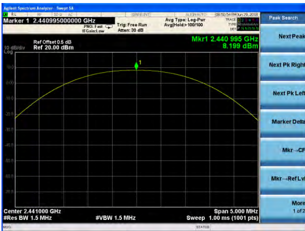
Peak output Power plot on channel 39 (1Mbps)
