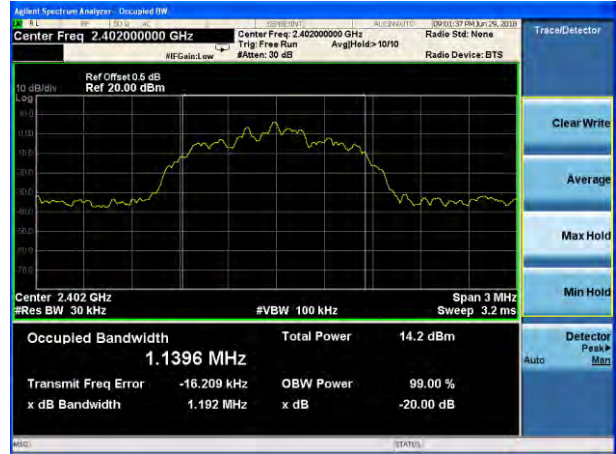
20dB Bandwidth plot on channel 39 (2Mbps)
