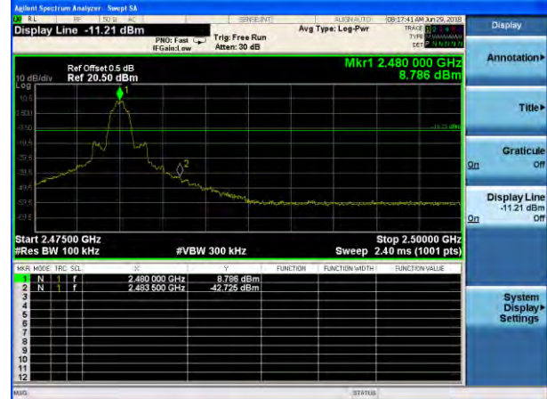
8-DPSK: Band Edge-High Channel
