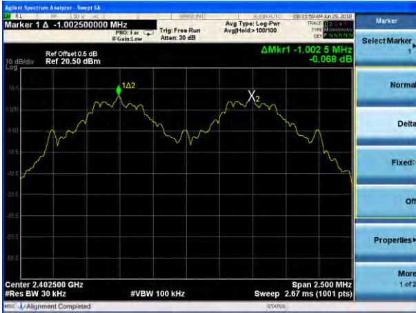
(1Mbps) Channel Separation plot on channel 39-40
