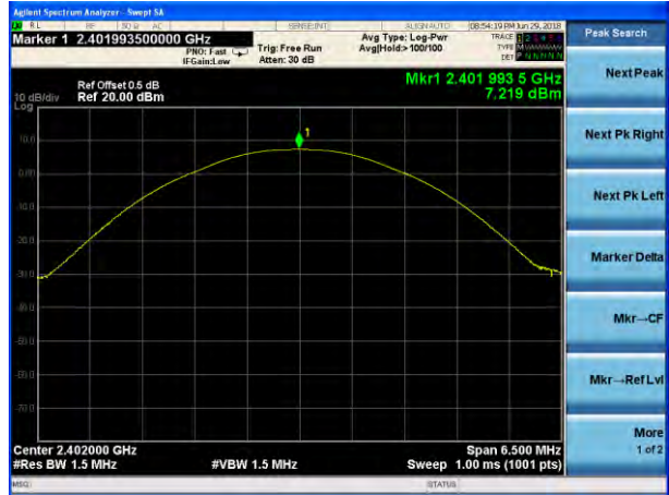
Peak output Power plot on channel 39 (2Mbps)
