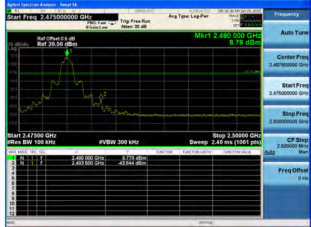
\pi /4-DQPSK: Band Edge-High Channel (Hopping Mode)
