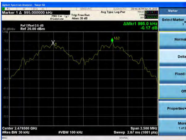
(1Mbps) Channel Separation plot on channel 77-78
