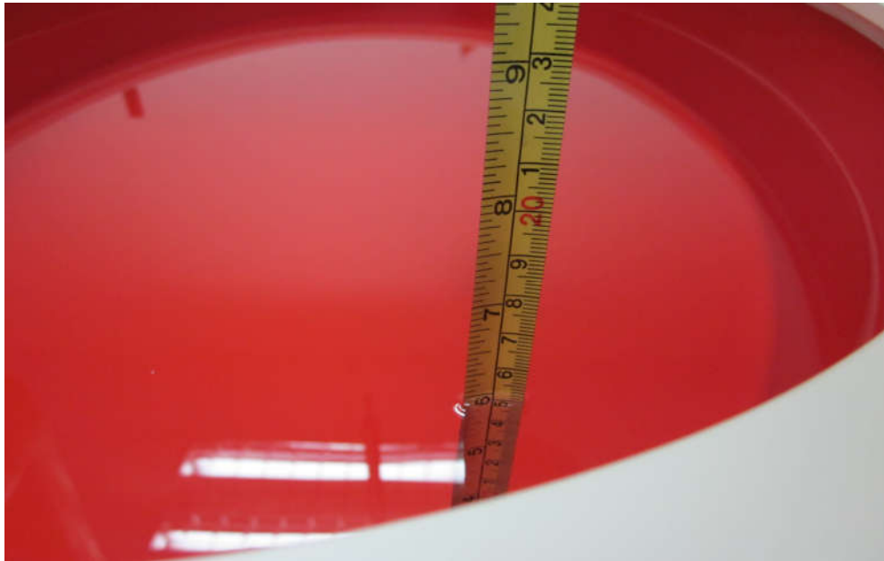
Figure 4.4: Liquid depth in the Flat Phantom
