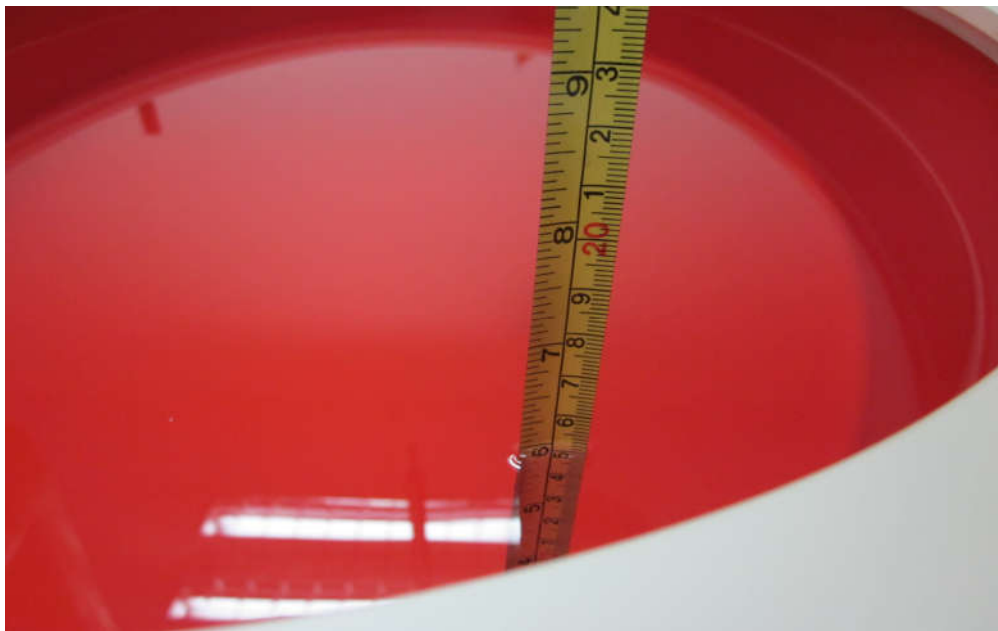
Figure 4.4: Liquid depth in the Flat Phantom
