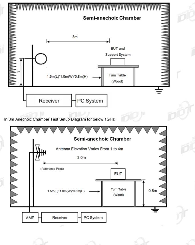
In 3m Anechoic Chamber Test Setup Diagram for frequency above 1GHz
