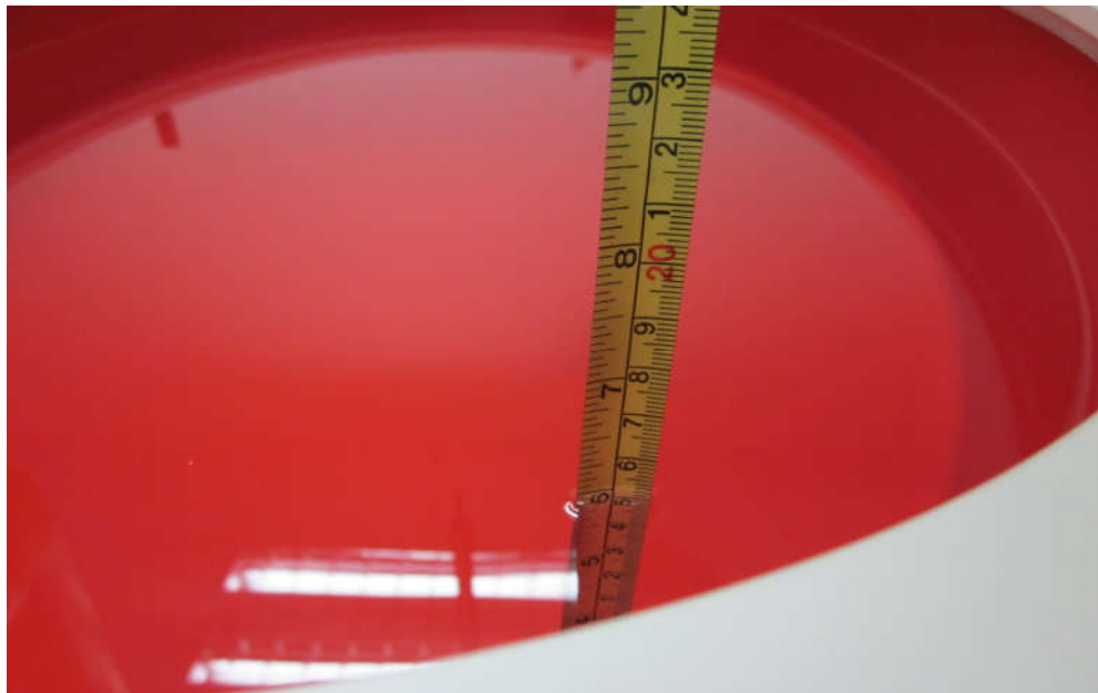
Figure 4.4: Liquid depth in the Flat Phantom
