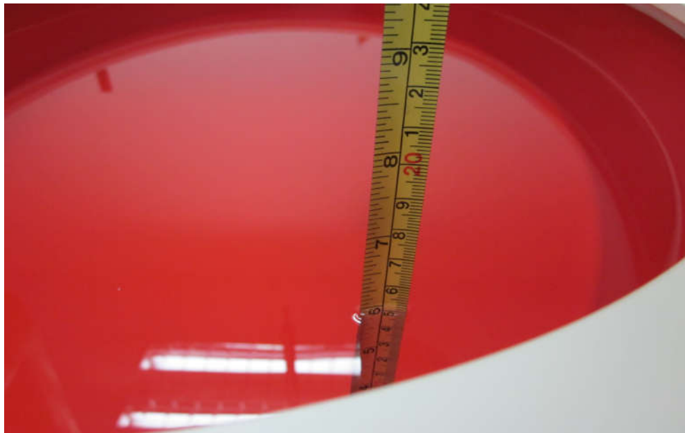
Figure 4.4: Liquid depth in the Flat Phantom
