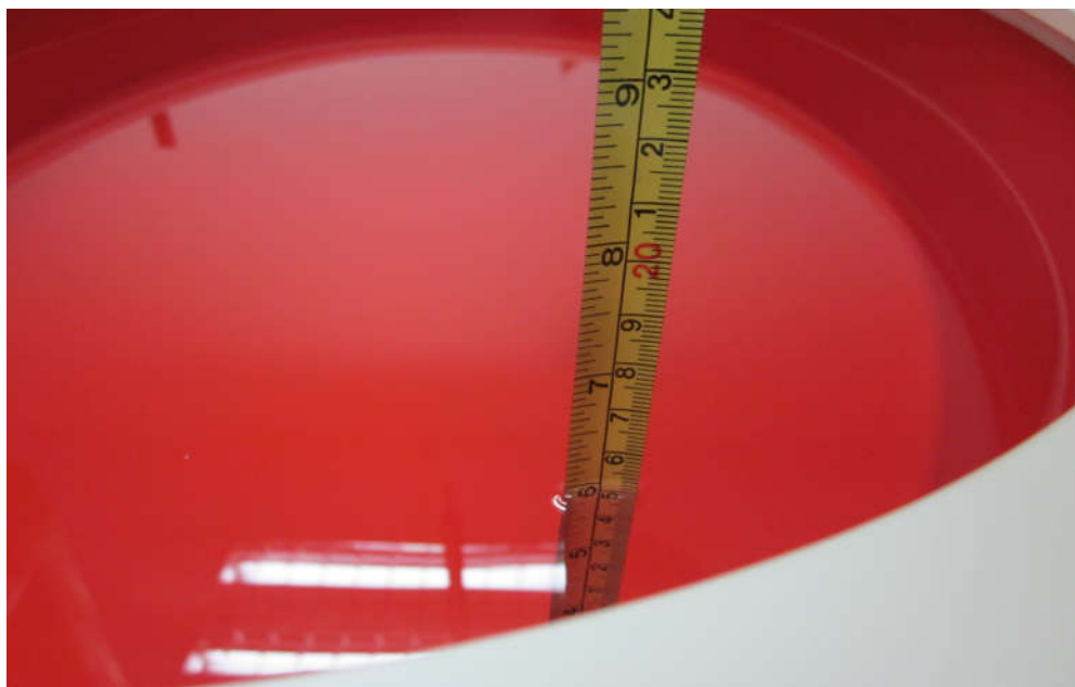
Figure 4.4: Liquid depth in the Flat Phantom
