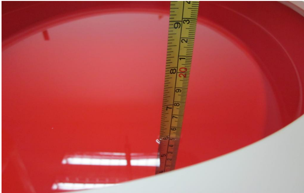
Figure 4.4: Liquid depth in the Flat Phantom
