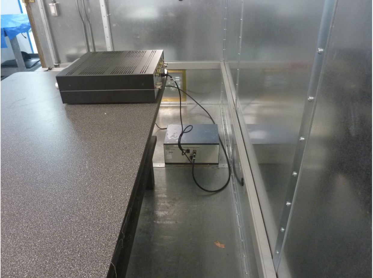
Figure 10: Conducted Emission Test Setup (Side)
