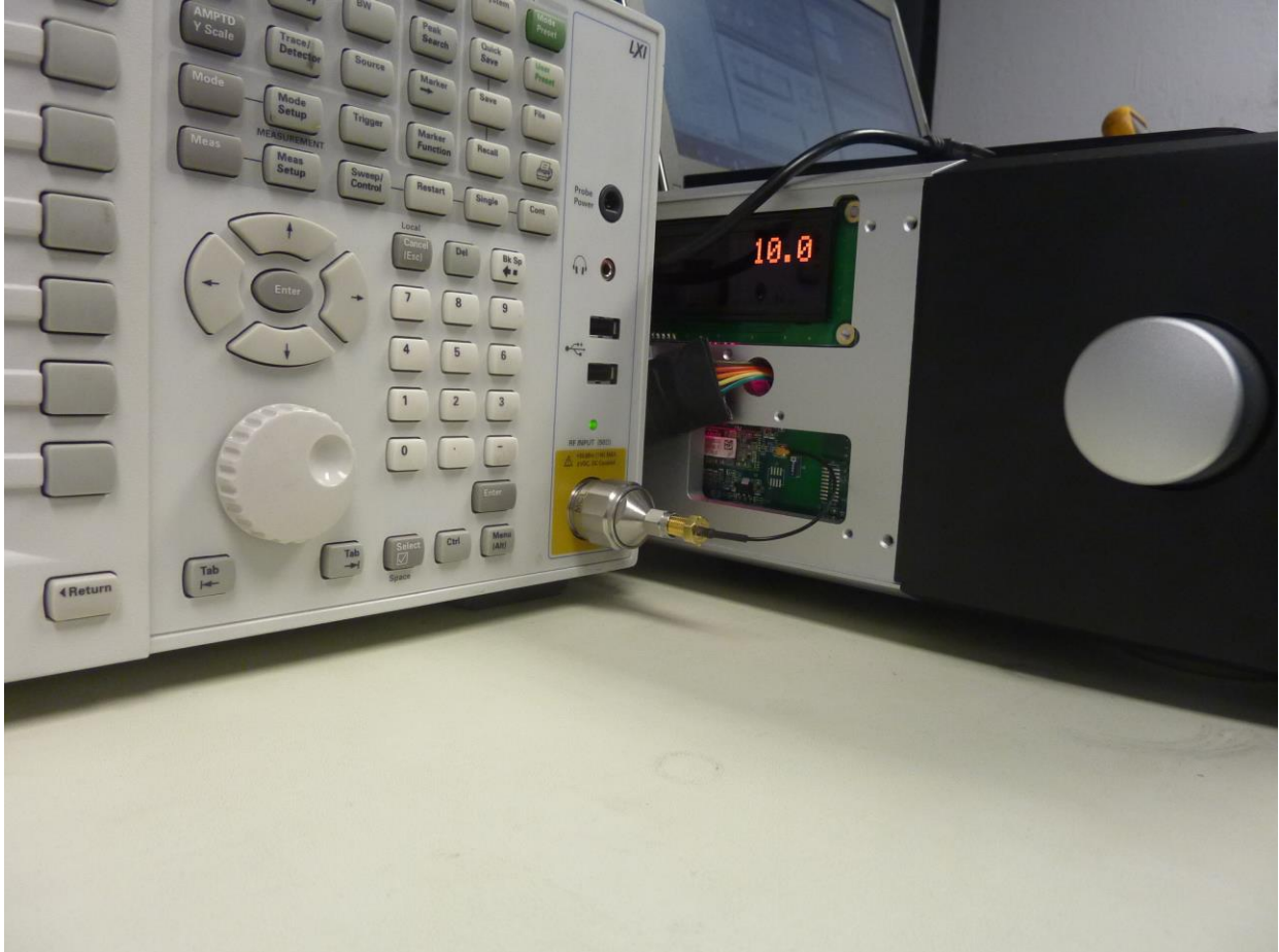
Figure 8: RF Conducted Test Setup – Closeup
