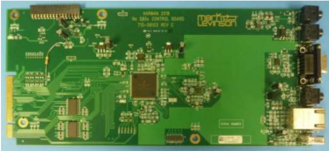
Figure 9: Photo of No5805 and No5802 Control PCB (Top View)
