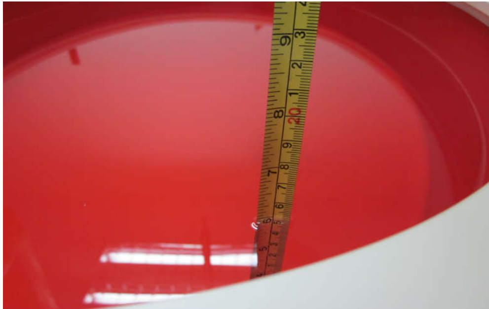
Figure 4.4: Liquid depth in the Flat Phantom
