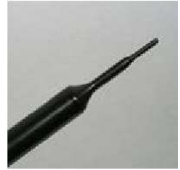
Figure 4.4 EX3DV4 E-field Probe
