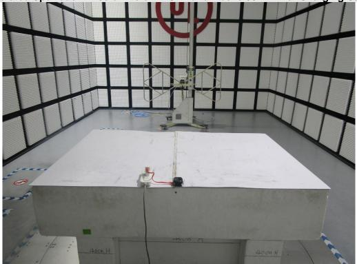
Radiated Spurious Emission Below 1 GHz and Above 30 MHz for Charging Case
