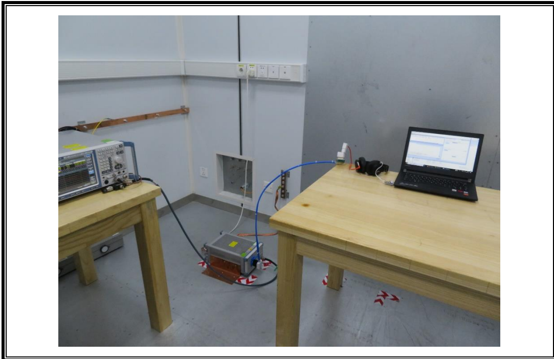
POWERLINE CONDUCTED EMISSIONS MEASUREMENT SETUP
