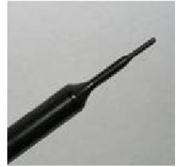
Figure 4.4 EX3DV4 E-field Probe
