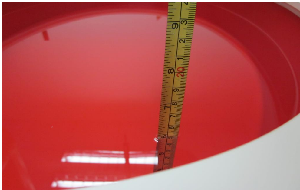
Figure 4.4: Liquid depth in the Flat Phantom
