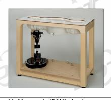
The shell corresponds to the specifications of the Specific Anthropomorphic Mannequin (SAM) phantom defined in IEEE 1528 and IEC 62209-1. It enables the dosimetric evaluation of left and right hand phone usage
