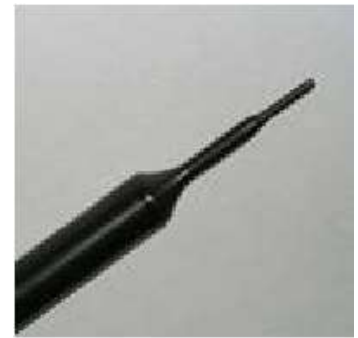
Figure 4.4 EX3DV4 E-field Probe
