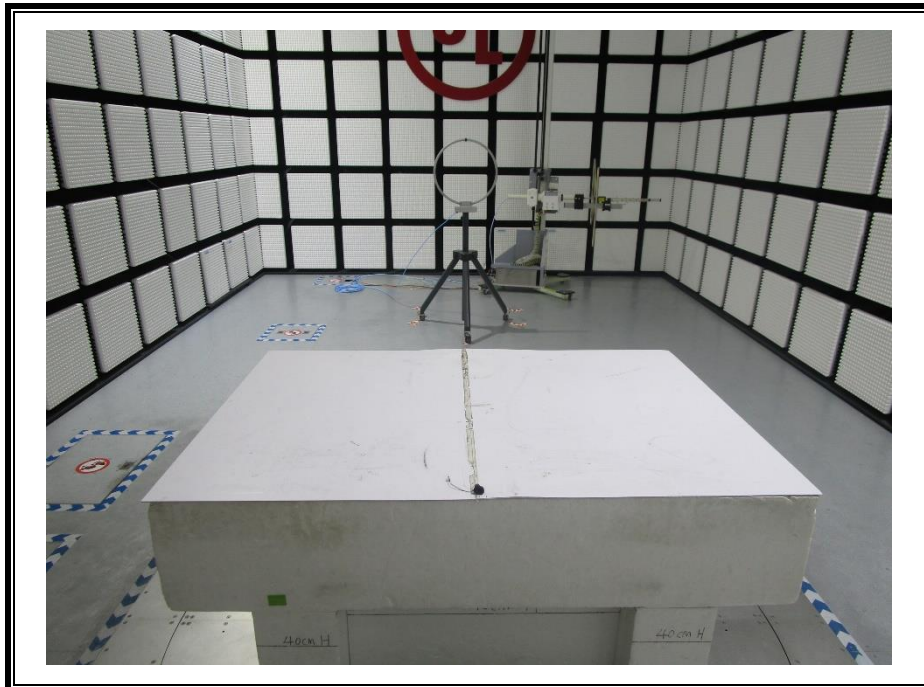
RADIATED RF MEASUREMENT SETUP (Below 30MHz)
