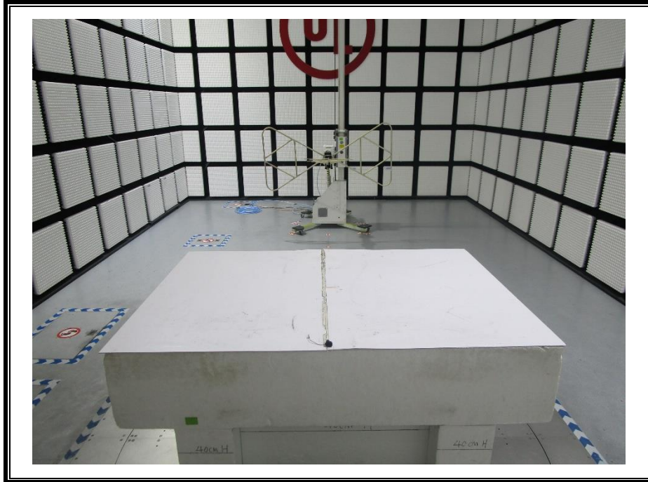
RADIATED RF MEASUREMENT SETUP (Below 30MHz)
