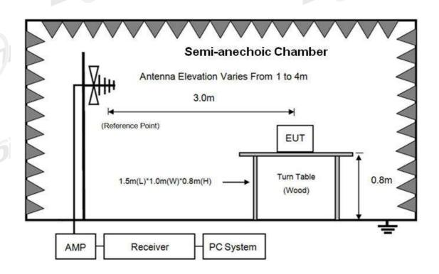
Semi-Anechoic 3m Chamber
