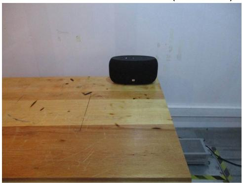
1.2 Radiated Spurious Emissions Test Setup
