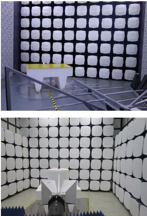
1.2 Radiated Spurious Emissions Test Setup
