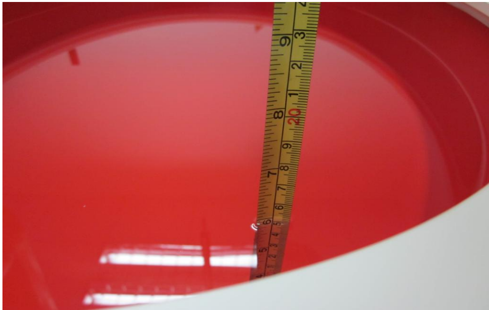
Figure 4.4: Liquid depth in the Flat Phantom
