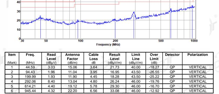
Note: 1. Result Level = Read Level + Antenna Factor + Cable loss.
