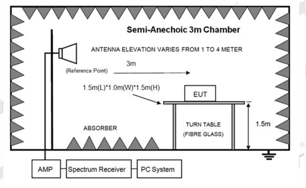
Note: For harmonic emissions test an appropriate high pass filter was inserted in the input port of AMP.
