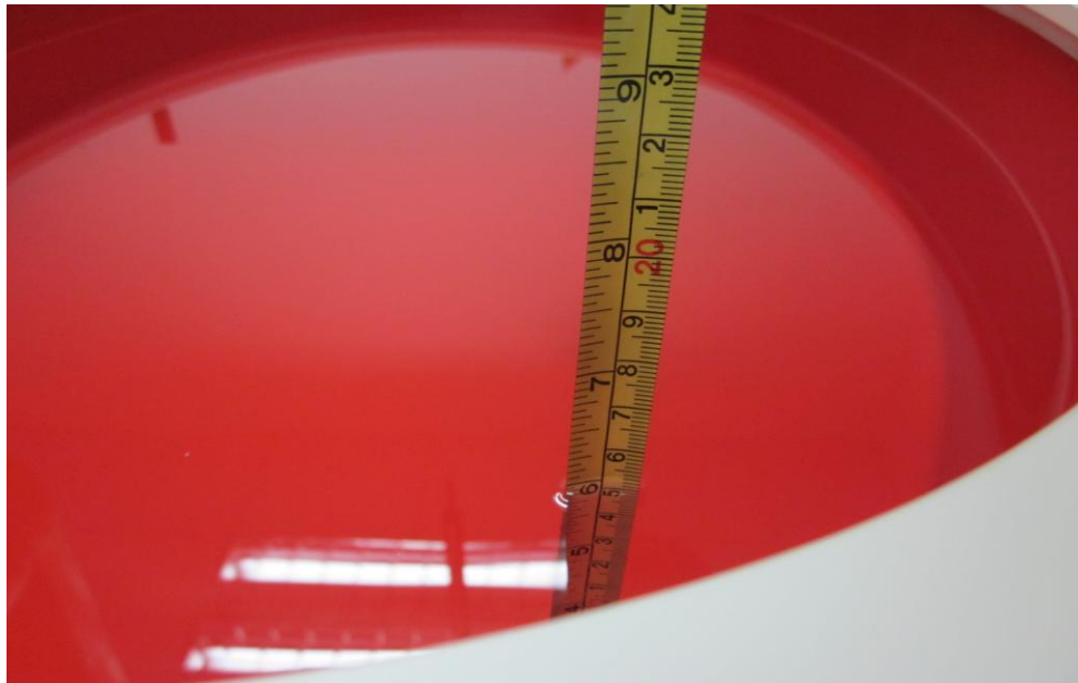
Figure 4.4: Liquid depth in the Flat Phantom
