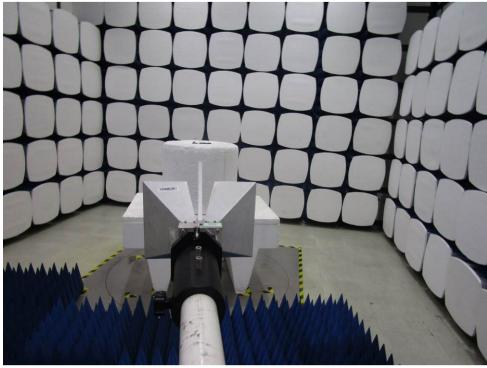
1.2 Radiated Spurious Emissions Test Setup
