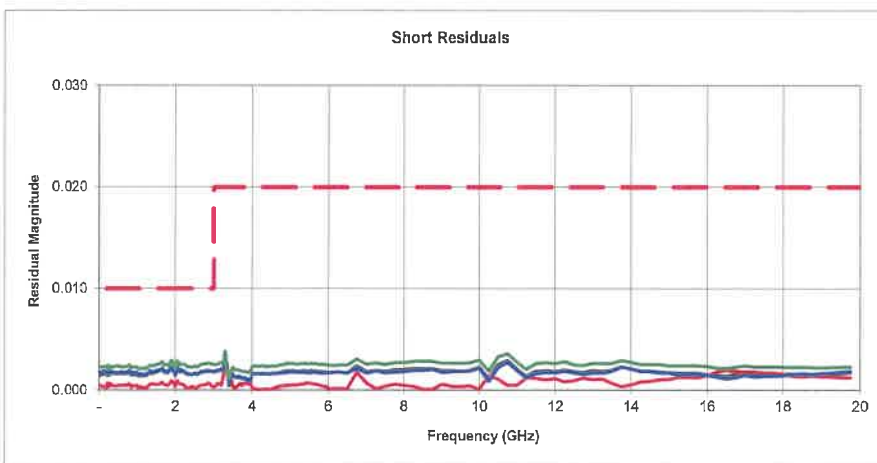
Fig. 2.1b Magnitude of the residual of the shorts, 200 MHz – 20 GHz, after calibration b)
