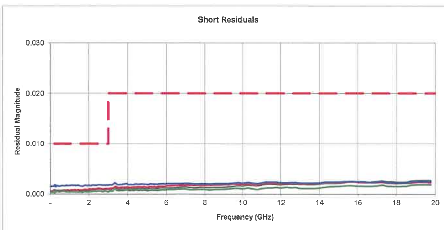
Fig. 2.1c Magnitude of the residual of the shorts, 200 MHz – 20 GHz, after calibration c)
