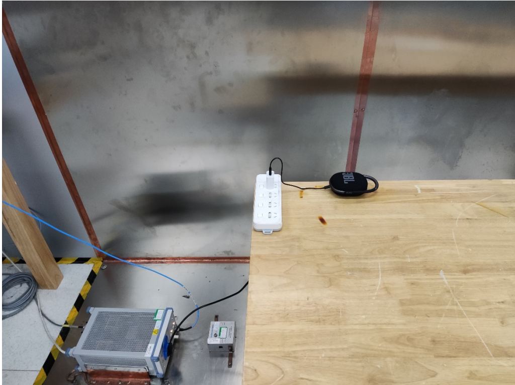
Photograph 3: Set-up for Conducted Emission on AC Mains
