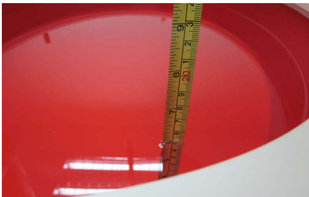
Figure 4.4: Liquid depth in the Flat Phantom
