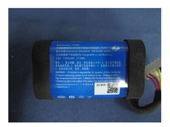
New Built-in battery model No: ID998-B
