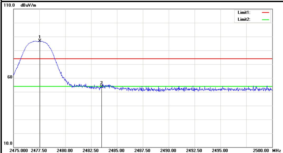
**Detector mode: Average****Polarity: Vertical**
